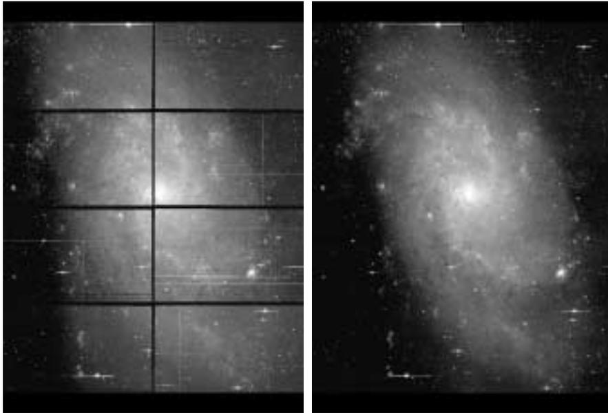
**Figure 2.** NOAO Mosaic CCD Camera pictures of M33 taken at the KPNO Mayall 4-meter. The left picture is a single 5 minute exposure showing the mosaic format of 8 CCDs each 2Kx4K for a full format of 8Kx8K. The right picture is a fully processed final image which is a combination of 5 dithered exposures. The processing was done using the MDHS data reduction software.
