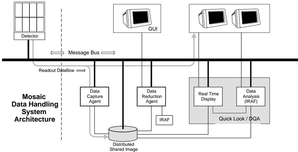
Figure 1. The Mosaic Data Handling System Architecture
